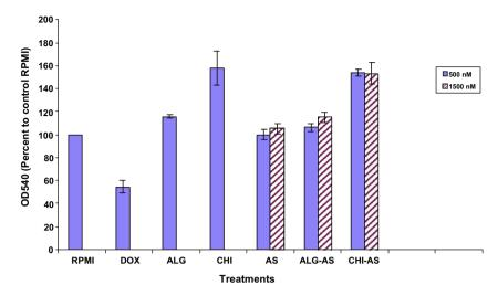
Fig. 1. Cytotoxicity of test compounds on T47D cells. The T47D cells were cultured in 96-well plates and exposed for 4 h to doxorubicin 250 nM, alginate and chitosan solution (50  $\mu$ g/ml), EGFR antisense alone (at two different concentrations 500 and 1500 nM), alginate and chitosan with two different concentrations of antisense (500, 1500 nM) and negative control of RPMI as explained in Section 2. All data are presented as mean of three different measurements  $\pm$  SE.
